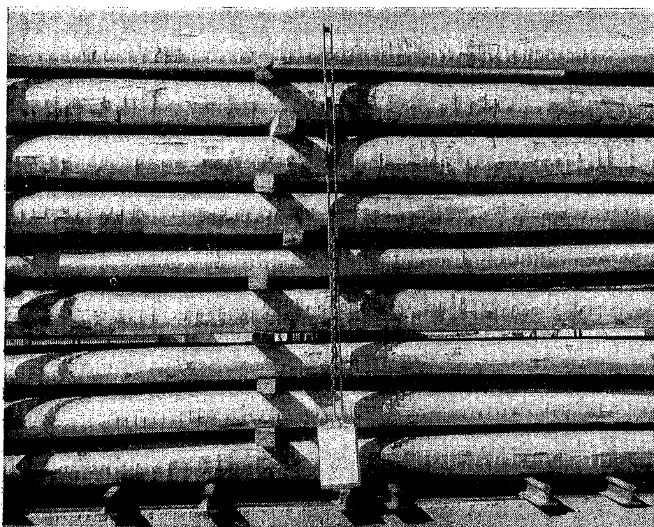
Fig. 2.—Typical appearance of P. radiata poles after drying for 81 hr at temperatures of up to 230°F.
