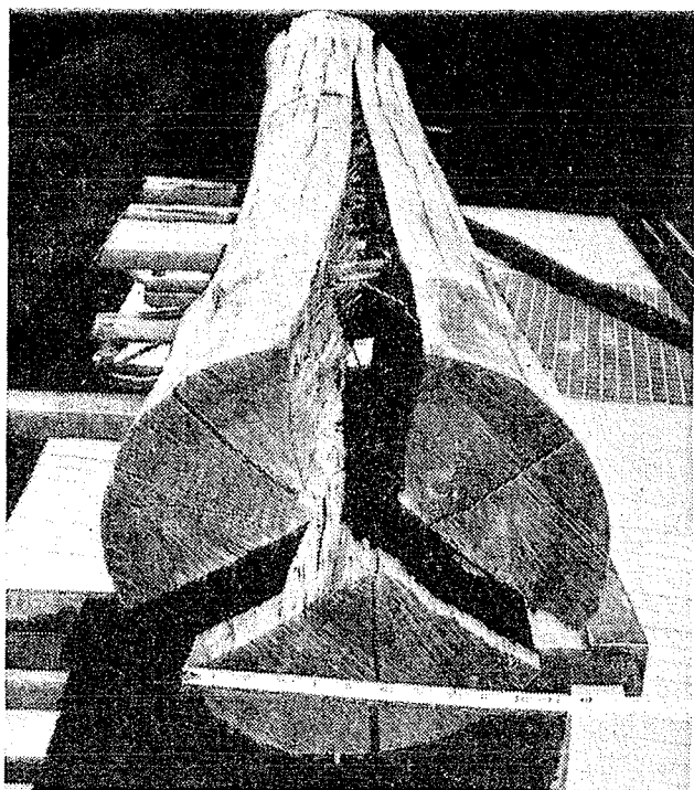
Fig. 1.—Air-dried karri specimen showing extremely severe end split and adjacent barrel checks.
